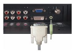
A digital signal that can support digital and convert analog to digital. DVI can be used for high resolution display and can support resolutions up to 1366 x 768.
