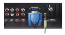
A standard graphic display system for computers that uses an analog signal and can support resolutions up to 1366 x 768.
